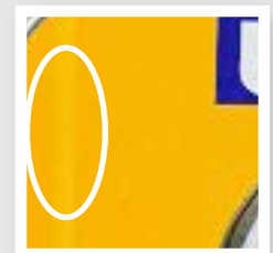
Detection of squeegee marks in a screen printing process.
