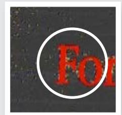
Detection of insufficient/excessive ink
